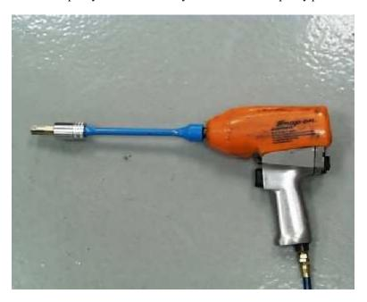
**Pros:** No investment in new special tools (unless you don't have a torque stick). Fast and easy. Works great for removal of old pulleys and works ok for installation if used with a torque stick.
