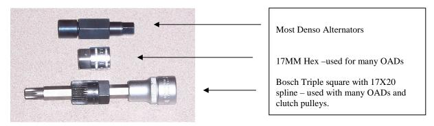
Note: There are other installation tools that are not show here. Always check to see what type of feature there is in the alternator shaft (10mm hex, 8mm allen, T50 torx, Triple square etc.) and match the tool accordingly. You will also need to match the correct tool to the clutch pulley/OAD shaft (17mm hex, 17x20 spline, 12x14 spline etc). If the alternator shaft does not have a feature in the end to allow you to turn it, then you will have to use method #2 or #3.
