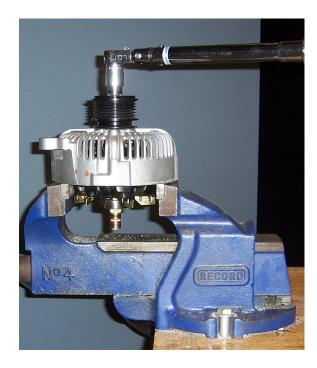
**Pros:** Correct installation torque can be achieved. It does not require the purchase of all of the special tools. Fast and easy if a total rebuild of alternator is being performed.
