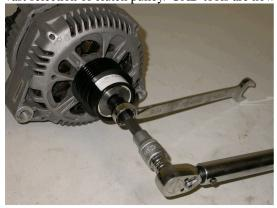
Some examples of the different types of Clutch pulley and Litens OAD installation tools.
